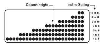
Diagram 7: Column height affected by changes in incline
